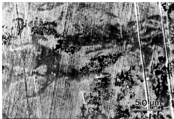
Figure 7 SEM micrograph of the worn surface of high-chromium iron at a load of 19.6 N.
